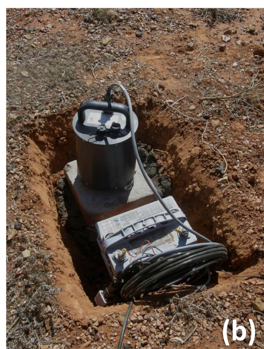
Above: Photographs of a typical field deployment site showing (a) trench for seismometer, (b) deployed seismometer, battery and GPS cables, (c) deployed and covered seismometer, (d) fully loaded field vehicle ready to head out, and (e) field vehicle with deployed seismometers at a deployment site.
