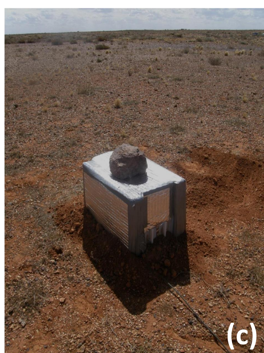
Above: Photographs of a typical field deployment site showing (a) trench for seismometer, (b) deployed seismometer, battery and GPS cables, (c) deployed and covered seismometer, (d) fully loaded field vehicle ready to head out, and (e) field vehicle with deployed seismometers at a deployment site.
