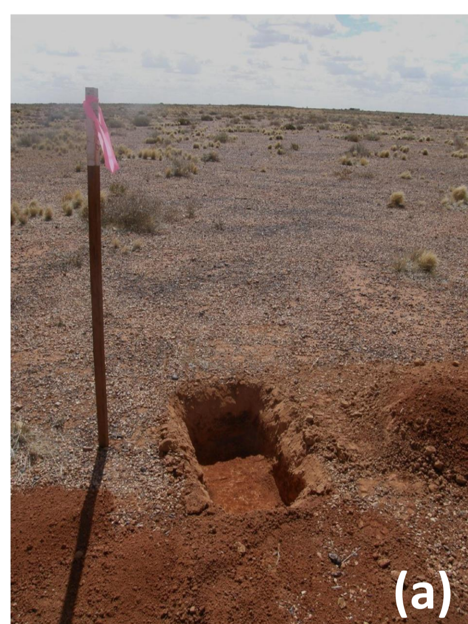
Above: Photographs of a typical field deployment site showing (a) trench for seismometer, (b) deployed seismometer, battery and GPS cables, (c) deployed and covered seismometer, (d) fully loaded field vehicle ready to head out, and (e) field vehicle with deployed seismometers at a deployment site.
