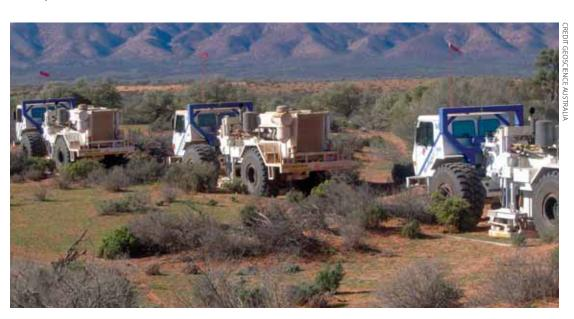
Seismic vibration machines, Flinders Ranges
