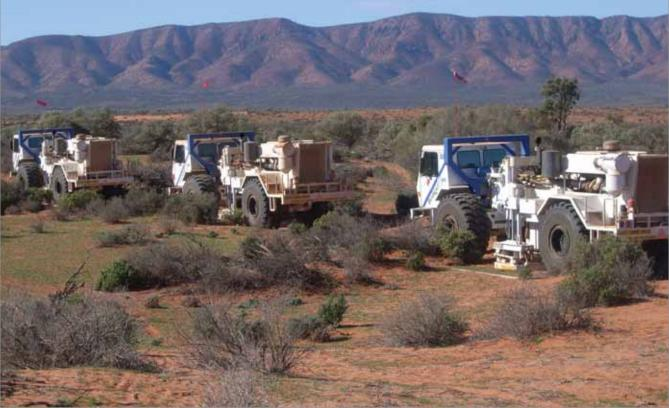
Seismic vibration machines assist in the search for resources deep within the Earth
