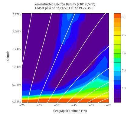
**Figure II.4.4:** Tomographically reconstructed density distribution using data recorded by the GPS receiver on FedSat. It shows an enhanced ionization plume moving upwards from the auroral region near 60 degrees southern latitude.
