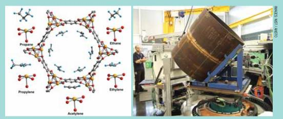
The first image is from *Science* 335(6076), 1606-1610 (2012), and is potentially important as a way to separate gases within natural gas streams without having to resort to energy-intensive liquefaction methods. It is part of a collaboration between UC-Berkeley, the National Institute of Standards and Technology and ANSTO.
