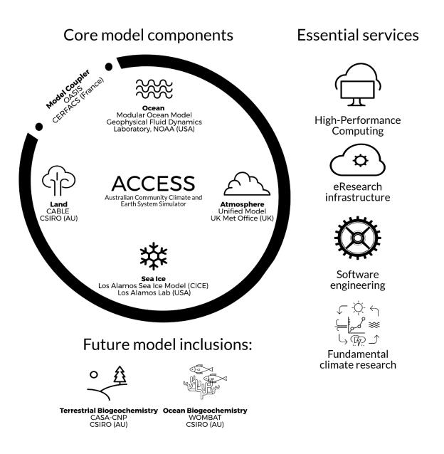
Figure 6. Australian Community Climate and Earth System Simulator (ACCESS) model, its components, and the essential services required for it to function.
