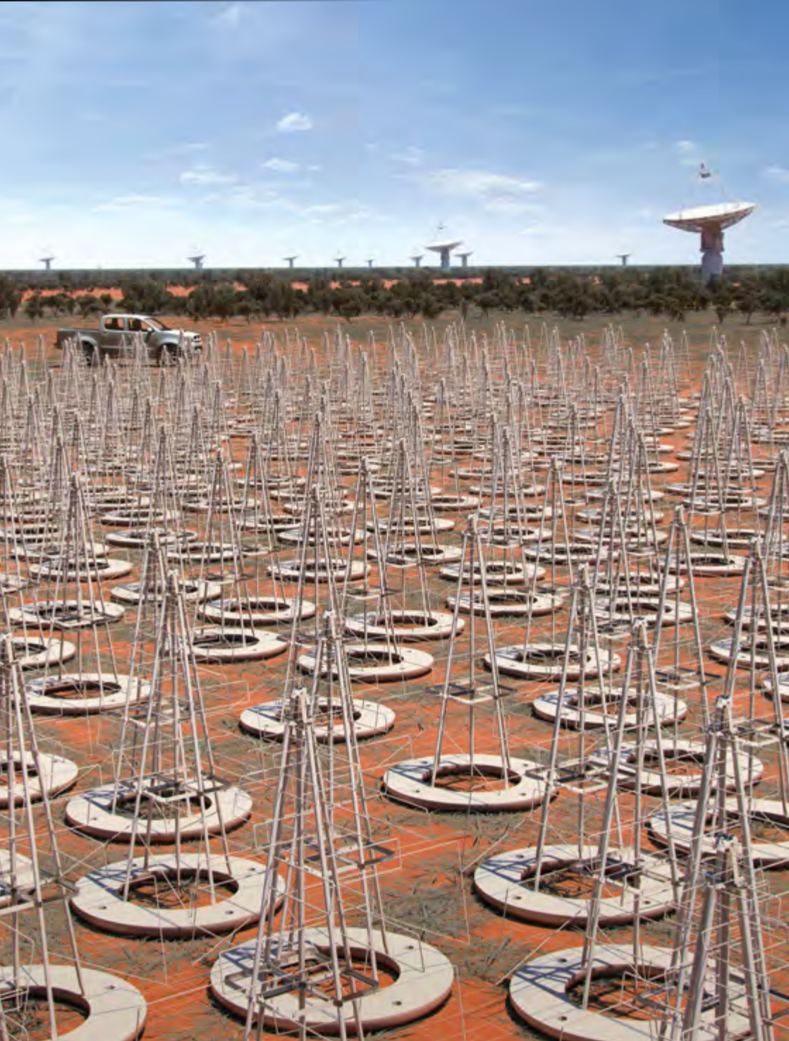
Artists impression of the SKA low frequency dipole antennas deployed at the MRO. CREDIT SKA ORGANISATION
