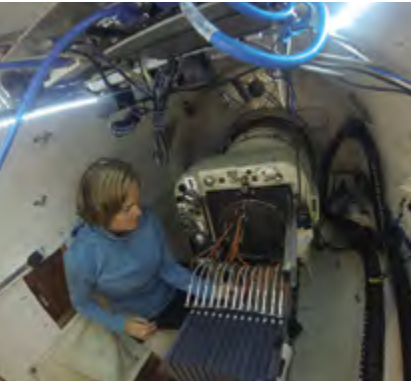
Preparing the the Sydney-Australian-Astronomical-Observatory Multi-object Integral-Field Spectrograph (SAMI) for observations on the AAT. SAMI allows a unique view of stars and gas inside distant galaxies by enabling collection of dozens of spectra across the entire face of each galaxy.
