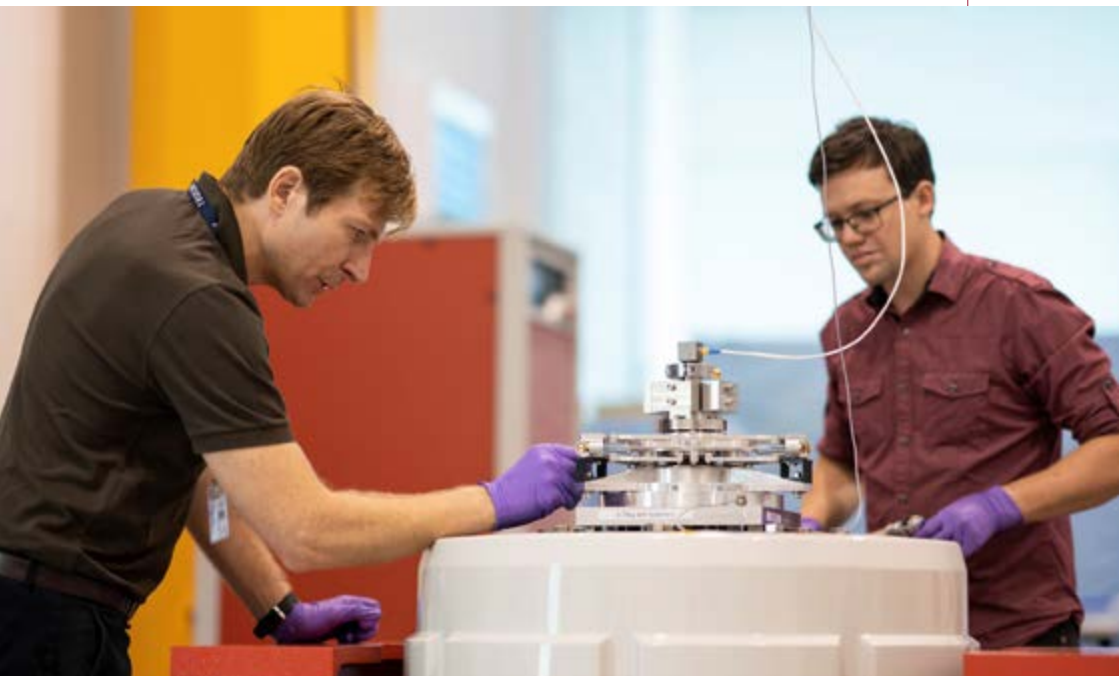
Eduardo Trifoni and David Adams work on a prototype anti-vibration mount at Mount Stromlo. Vibration is a big challenge for future telescopes, and engineers at ANU are creating new solutions to this difficult problem. CREDIT: LANNON HARLEY, ANU
