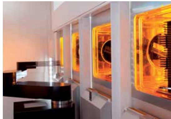
A commercial, high-volume ion implantation instrument for semiconductor manufacture. Image courtesy Applied Materials.
