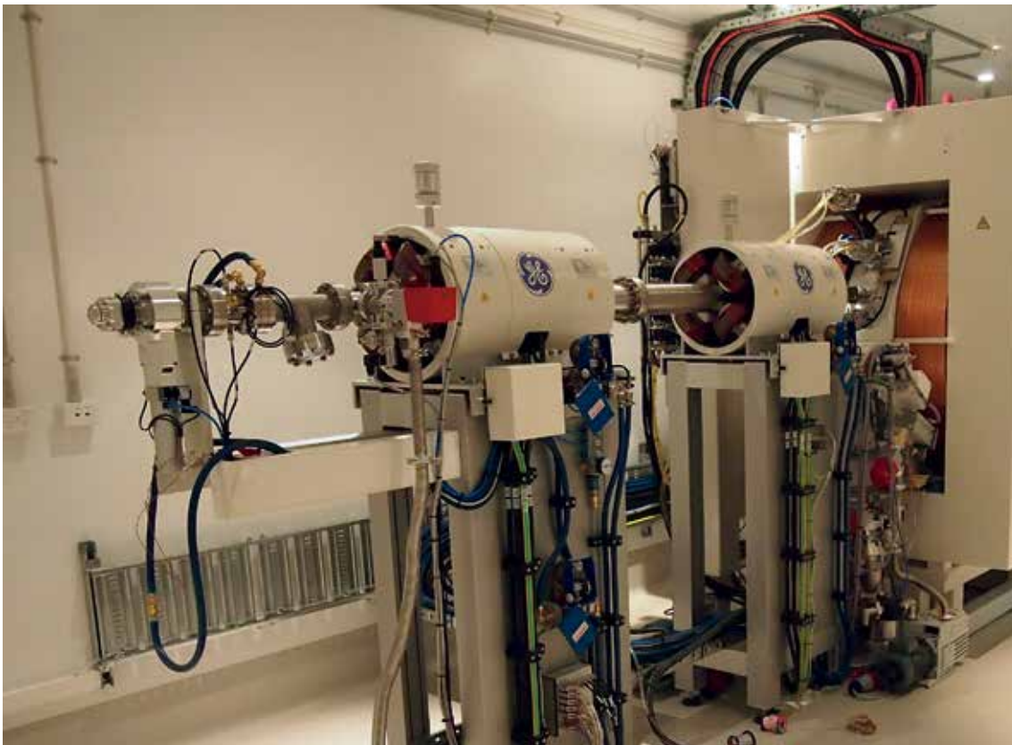
A GE medical cyclotron that accelerates protons to produce radioactive isotopes for PET imaging. Image courtesy South Australian Health and Medical Research Institute.
