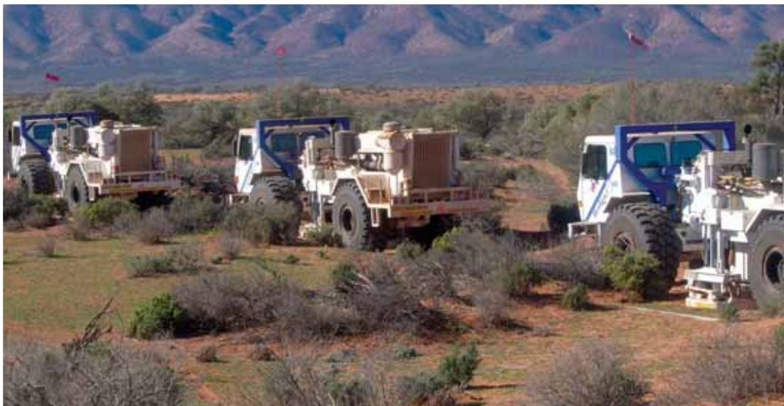
Seismic vibration machines, Flinders Ranges
