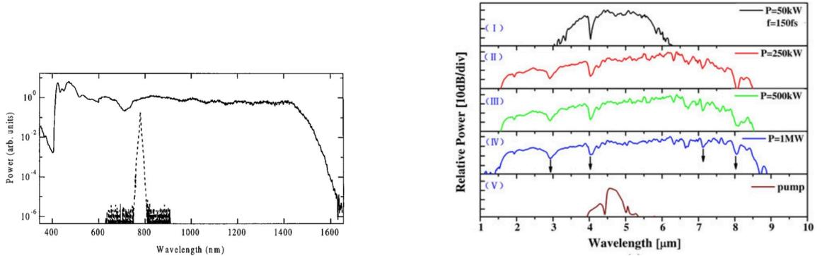
Figure 12: Left: spectrum of the input 770 nm 100 fs, 1.6 kW input pulse (dashed) and the output power from a MOF [68]. Copyright OSA. Right: Experimental SC spectra with different pump peak powers from a  $\text{As}_2\text{Se}_3$ – $\text{As}_2\text{S}_3$  chalcogenide glass fibre in the mid infrared (from [70]). Copyright IEEE.
