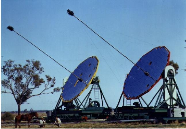
Figure 8: The mosaic mirrors on their carriages at the Narrabri stellar interferometer.(Figure copyright: University of Sydney).
