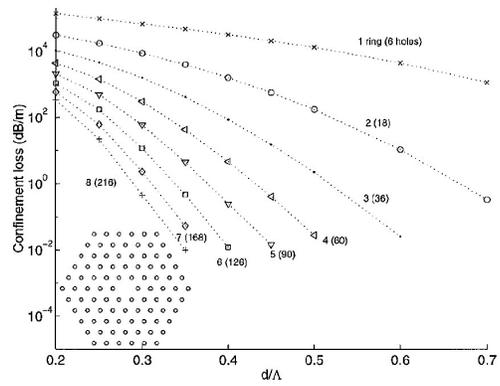
Figure 11: Left: the structure of a microstructured fibre (figure courtesy of H. Kubota). Right: confinement loss in a microstructured fibre of air holes with diameter to spacing ratio  $d/\Lambda$  in silica as a function of the number of rings in the hexagonal structure.
