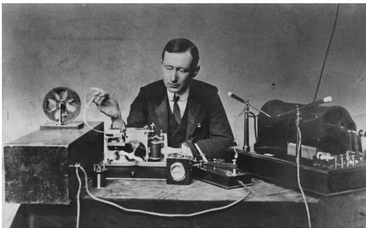
Figure 1: Marconi with the equipment used for long-distance transmission in the 1890's. The transmitter is at right, with the receiver and paper tape printer at left. (LIFE Photo Archive: 4a204d82f07524bd.)
