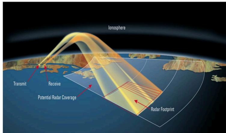
Figure 13: Left: Geographic coverage of the JORN network (copyright Wikimedia Commons: CC BY-SA 3.0). Right: operating principle of JORN (copyright JORN OTHR Operating Principles.RAAF).
