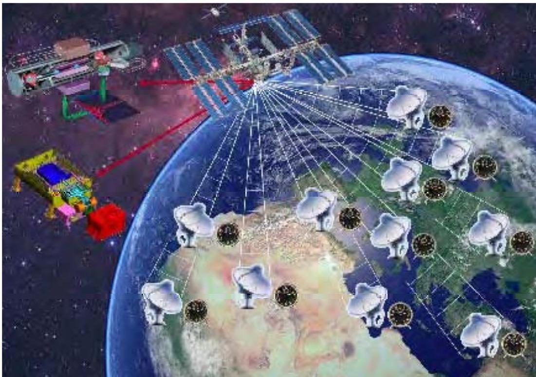
Figure II.4.11: The ACES mission. Ultra-stable atomic clocks on-board the International Space Station are compared to a network of ground clocks through a high performance two-way time transfer system
