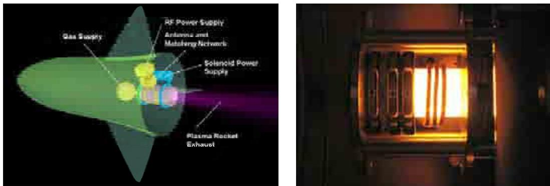
Figure II.4.10: Plasma thruster (left) concept and (right) device.
