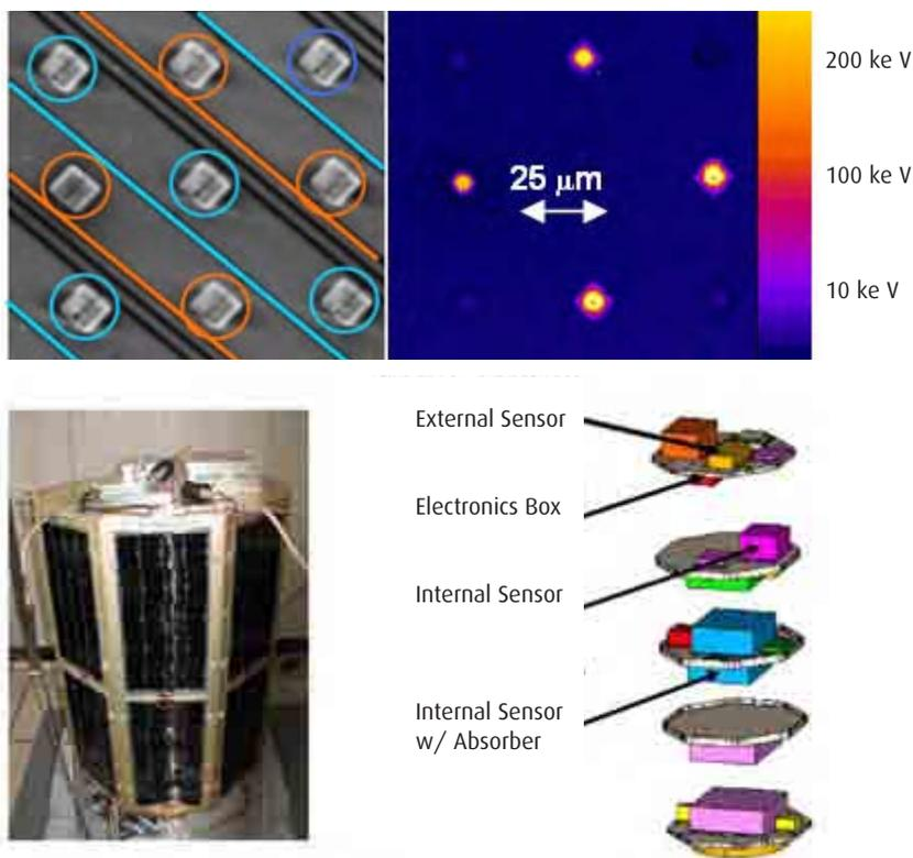
Figure II.4.12 (Top) (Left): Fragment of a CMRP microdosimeter chip and (right) the energy deposited on cellular scales by 3 MeV alpha particles. (Bottom): CMRP microdosimeters installed in the MIDN instrument inside and outside the 2007 US MidSTAR satellite, to investigate radiobiological effects in Low Earth Orbit. Collaborative research with US Naval Academy supported by NASA.
