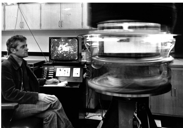
Fig. 1. Dr Angus McEwan and his 'rotating table' at the CSIRO Aspendale laboratory, around 1980. Fluid experiments are performed on such rotating tables in order to simulate the effects of the rotation of planet earth on fluid motions.
