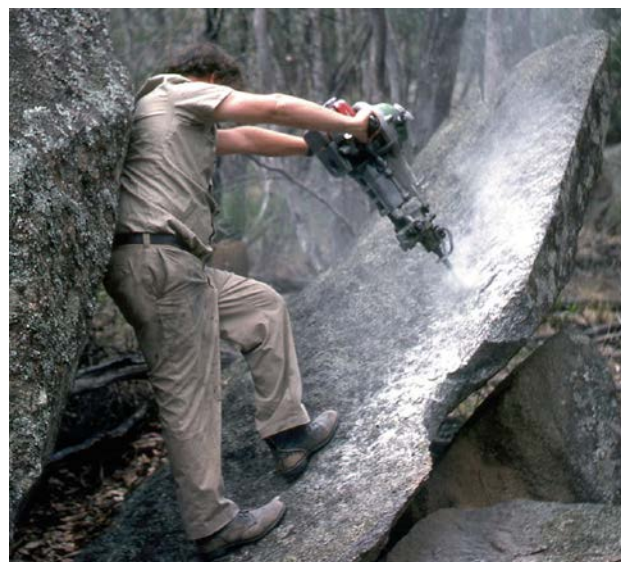
Figure 4. Collecting granite at Moonbi in 1975. Rocks too large to be broken with a sledge hammer were drilled, then split with feathers and wedge. Samples for whole rock geochemistry commonly weighed in excess of 20 kg.
