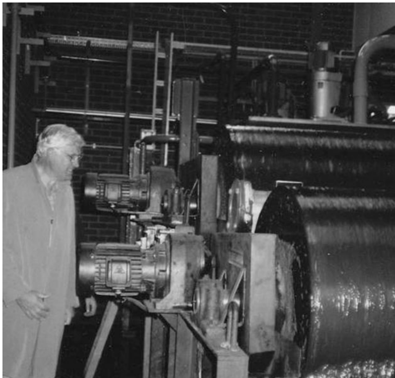
Figure 3. Don Weiss inspecting the Sirofloc magnetic regeneration train at Bell Bay.
