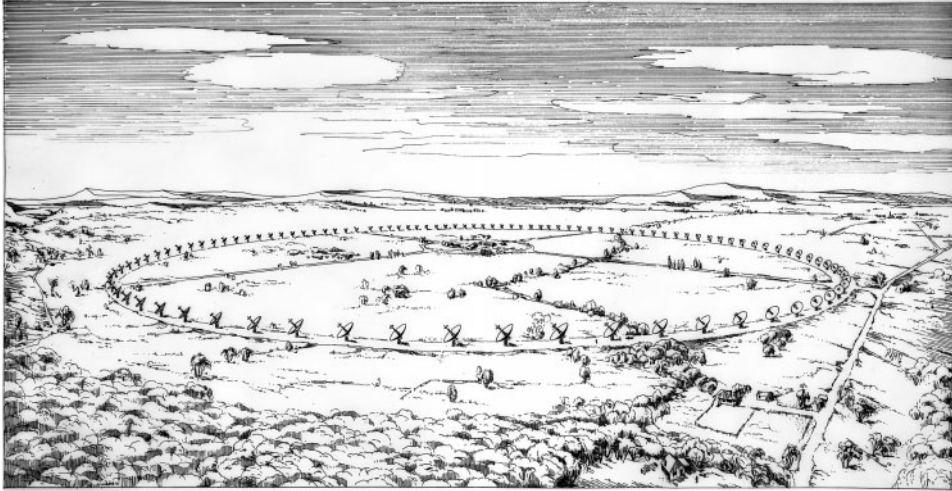
Figure 2. Artist's impression for the Radio Heliograph built at Culgoora near Narrabri in north-west NSW in 1967. The 96 13.7 m dishes evenly placed in a circle 3 km in diameter. © CSIRO Australia.
