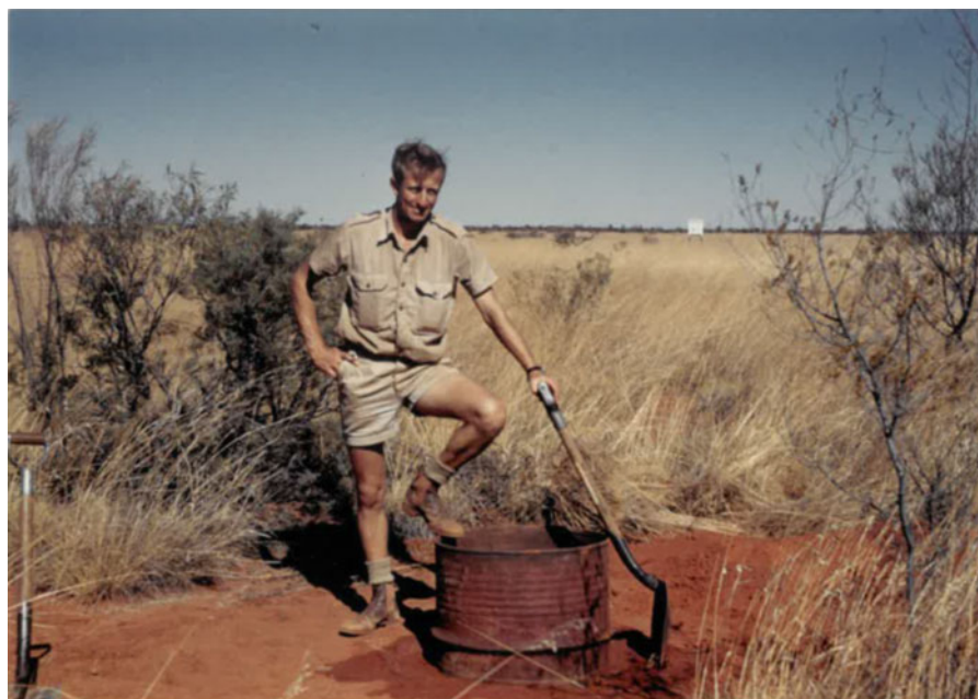
Figure 2. CSIRO Water infiltration experiment ‘60 mile’ Spinifex site, Alice Springs, 1959 (photograph from Slatyer collection, published with permission of Dr Chin Wong).
