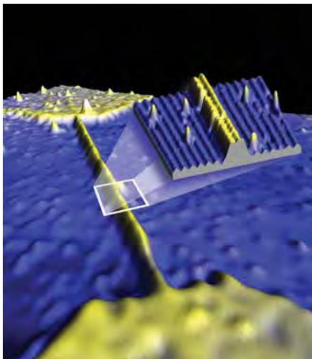
**Figure 34:** Researchers at UNSW have created the world's thinnest nanowire in silicon, just a few phosphorus atoms wide, and demonstrated that it still has a high conductivity. (Image courtesy of Bent Weber, UNSW)
