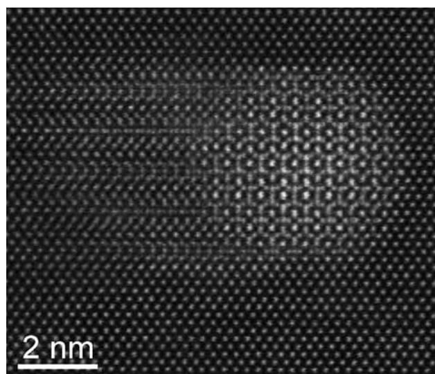
**Figure 6:** Image of the arrangement of atoms in a tin nano particle attached to an aluminium copper nano particle embedded in an aluminium alloy developed for high performance structural applications taken with a double-aberration-corrected TEM. (Reprinted from *Acta Materialia*, Bourgeois, L *et al.* (2012) The magic thicknesses of theta prim-prime precipitates in Sn-microalloyed Al-Cu, 60: 633–644 with permission from Elsevier; Image courtesy of Laure Bourgeois, Monash University)
