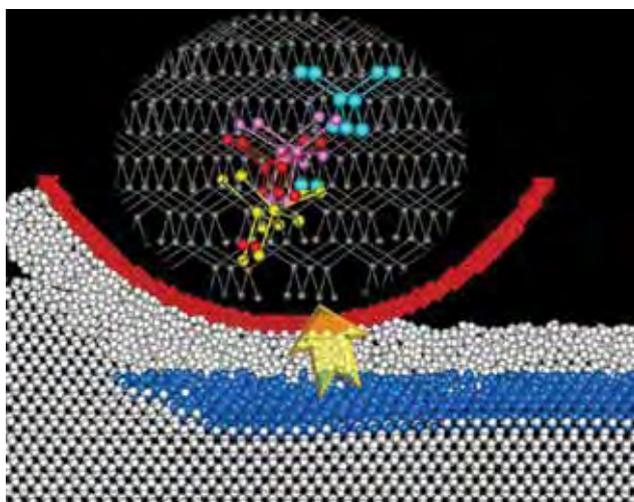
**Figure 46:** A nanomanufacturing process to create functional, layered microstructures of distinguished electronic properties in silicon. The layers showing from top to bottom are amorphous silicon, bct-5 silicon (in blue) and diamond silicon, respectively. (Image courtesy of Liangchi Zhang, UNSW)
