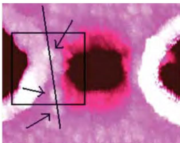
**Figure 36:** Researchers at CSIRO have used a Nb nano-SQUID pictured here (the central nanoSQUID hole is about 150 nm across) to detect the magnetism of single nanoparticles of native horse-spleen ferritin (location indicated by the arrows). (Image courtesy of Simon Lam, CSIRO)
