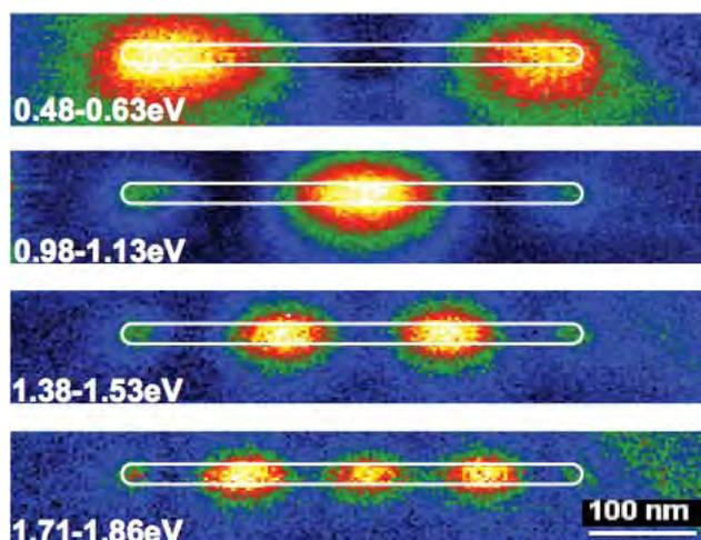
Figure 11: Silver nanoantennas. Using latest advances in TEM, surface plasmon-polariton resonances can be detected at nanometre resolution in individual antennas. (Reprinted from *Nano Letts* (2011) 11:1499–1504 with permission from ACS Publications; Image courtesy of the Canadian Centre for Electron Microscopy, McMaster University).
