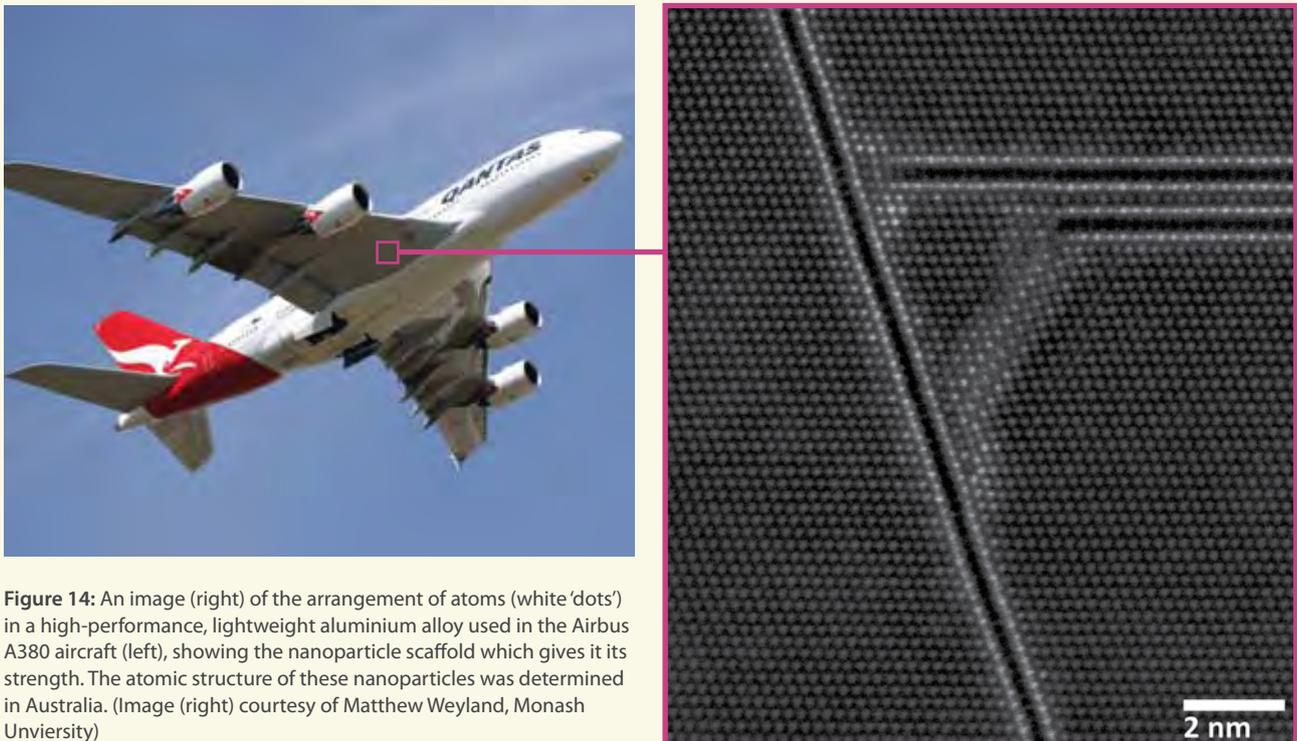
**Figure 14:** An image (right) of the arrangement of atoms (white 'dots') in a high-performance, lightweight aluminium alloy used in the Airbus A380 aircraft (left), showing the nanoparticle scaffold which gives it its strength. The atomic structure of these nanoparticles was determined in Australia. (Image (right) courtesy of Matthew Weyland, Monash University)
