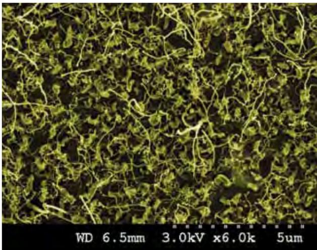
**Figure 30:** Glass 'nanowool' made by ion implantation. (Image courtesy of ANU)
