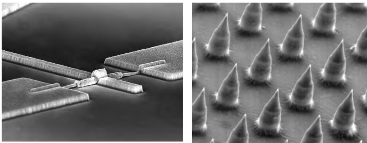
**Figure 18:** Examples of lithography and etching techniques. (Left) Semiconductor nanowire with electrodes patterned by electron-beam lithography. (Image courtesy of Adam Micolich, UNSW and Kristian Storm, Lund). (Right) Silicon microneedles fabricated using reactive ion etching. (Image courtesy of ANFF, University of Queensland)
