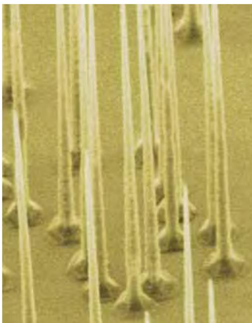
**Figure 26:** Semiconductor nanowires for optoelectronics. (Image courtesy of ANU)
