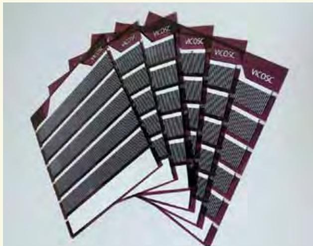
**Figure 39:** Fully printed solar cells. (Image courtesy of the Victorian Organic Solar Cell Consortium)
