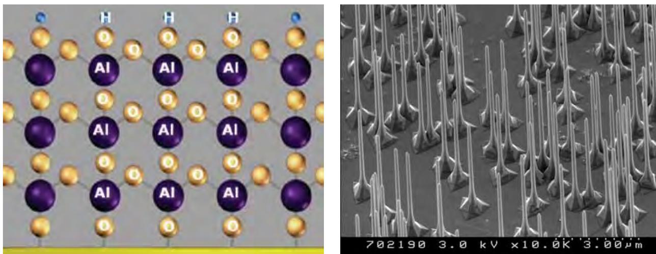
**Figure 17:** Examples of growth and deposition techniques. (Left) Growth of thin film using atomic layer deposition, (Image courtesy of Cambridge nanotech). (Right) III-V compound semiconductor nanowire growth. (Image courtesy of ANFF, ANU)
