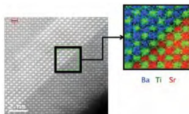
Figure 12: Atomic resolution chemical maps of a BaTiO<sub>3</sub>/SrTiO<sub>3</sub> interface for functional electronics using the electron energy-loss signal from a next-generation aberration-corrected, monochromated TEM. Australian researchers contributed to the theoretical interpretation. (Reprinted from *Ultramicroscopy* 110, 926 (2010) with permission from Elsevier; Image courtesy of the Canadian Centre for Electron Microscopy, McMaster University).
