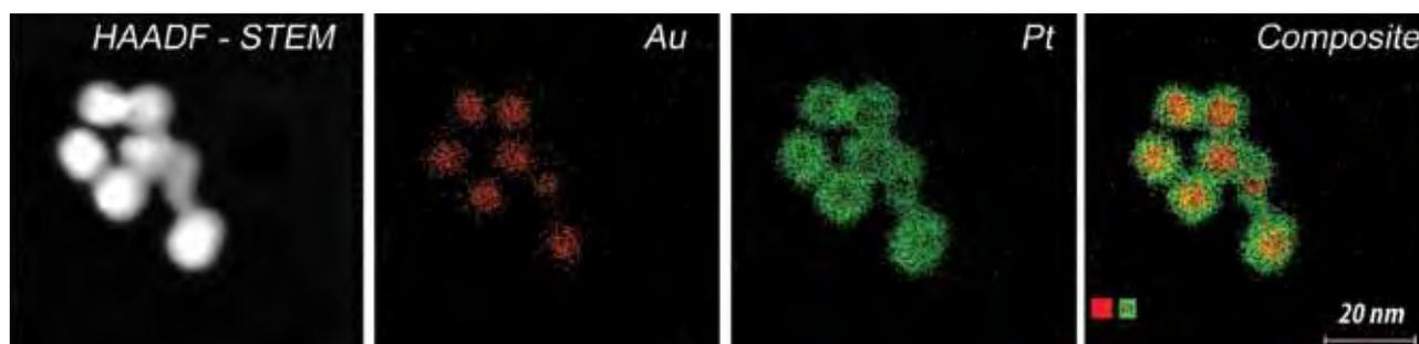
**Figure 5:** Electrocatalyst core/shell Au/FePt<sub>3</sub> nanoparticles for use in membrane fuel cells. Maps of the chemical distribution in the nanoparticles using X-ray spectroscopy in a TEM: of Au (green), Pt (red) and their overlap. (Similar material published in *Nano Lett.* (2011) 11: 919-926; Image courtesy of Nestor J Zaulzec)
