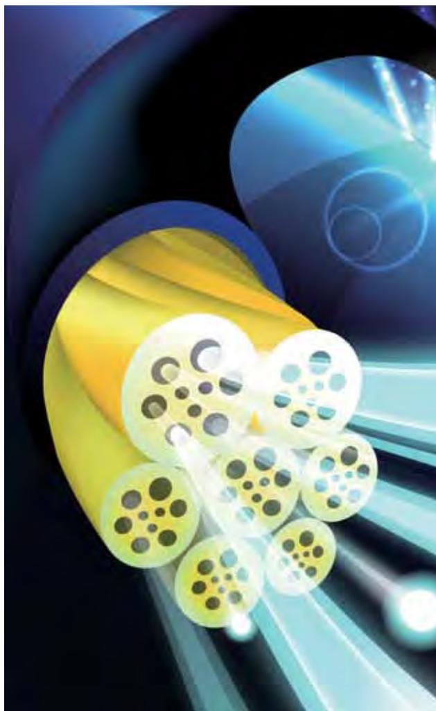
**Figure 35:** Schematic of nanoscale carbon doped magnesium diboride superconducting multifilament wires, which currently hold the world record in critical current carrying capacity, fabricated at the Institute for Superconducting and Electronic Materials. (Image courtesy of S. X. Dou, University of Wollongong)
