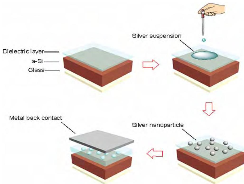
**Figure 37:** Increasing the efficiency of thin-film nanoplasmonic solar cells to a new world record by integration of silver nanoparticles into amorphous silicon solar cells. (Reprinted from *Nano Letts* (2012) 12: 2187-2192; Image courtesy of M. Gu, Swinburne University of Technology)
