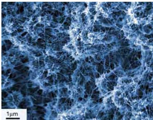
Figure 24: Boron nitride nanotubes. (Image courtesy of ANU)
