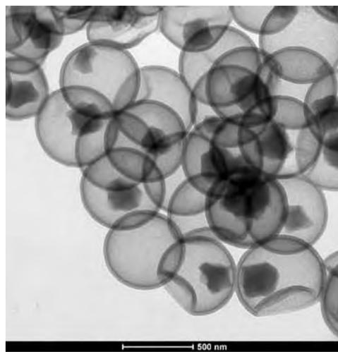
**Figure 29:** Silica hollow sphere for O<sub>2</sub> delivery to cell. (Image courtesy of Rose Amal, UNSW)
