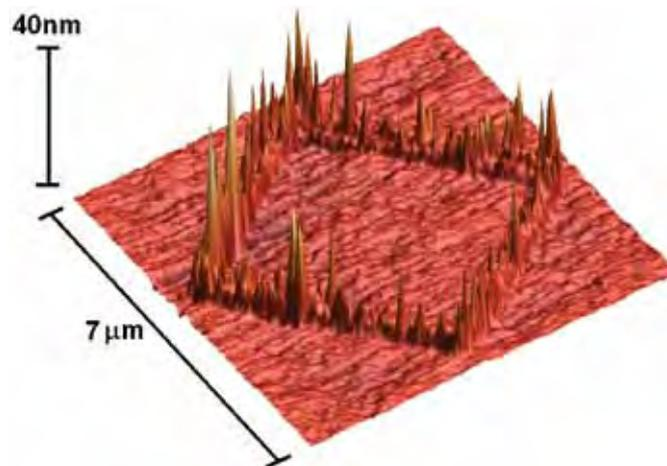
**Figure 8:** AFM Image of Patterned attachment of nanotubes to silicon created using AFM lithography. Reprinted from *Soft Matter*, Flavel B S *et al.* (2009) Patterned Polyaniline & Carbon Nanotube/Polyaniline Composites on Silicon, 5: 164 – 172; Image courtesy of Joe Shapter, Flinders University)
