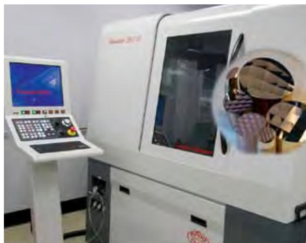
**Figure 47:** The ultraprecision machining centre installed at UNSW is capable of manufacturing large surfaces of up to 0.35 m in diameter but with functional features of submicron accuracy. The insert demonstrates a series of manufactured aspherical lens arrays. (Image courtesy of Liangchi Zhang, UNSW)
