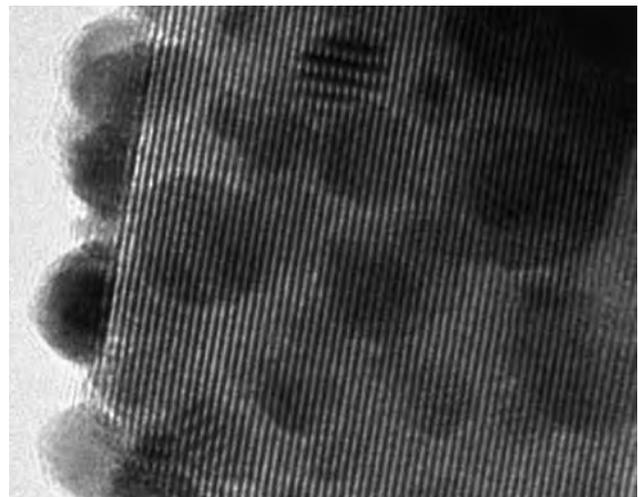
**Figure 31:** Gold seeded magnetite for highly sensitive environmental sensing. (Image courtesy of Rose Amal, UNSW)
