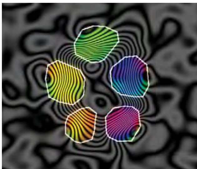
Figure 13: Magnetic field distribution in magnetic nanoparticle arrays measured using electron holography. The scale bar is 20nm. (Reprinted from *Nature Materials* (2009) 8: 271-280; Image courtesy Rafal E. Dunin-Borkowski)
