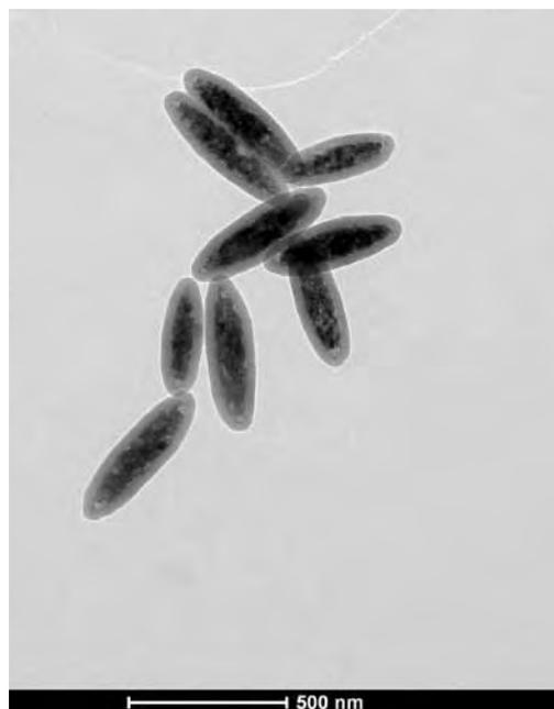
**Figure 27:** Ellipsoidal silica-coated magnetite for enhanced ultrasound imaging. (Image courtesy Rose Amal, UNSW)
