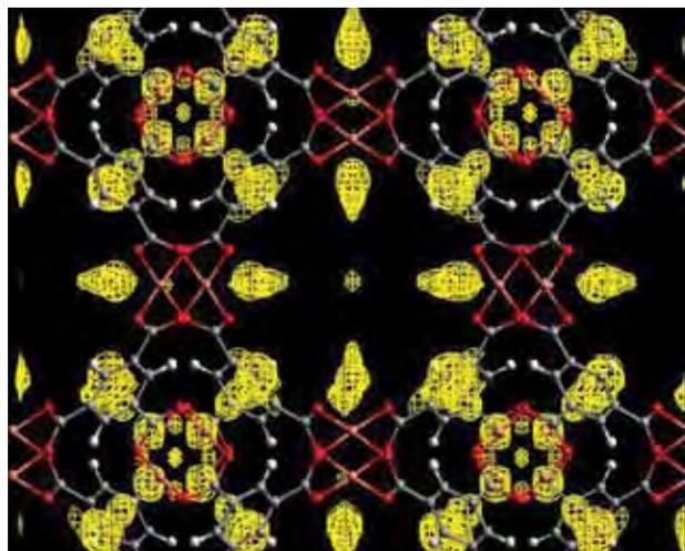
**Figure 4:** Nanoporous metal-organic framework containing molecular hydrogen (yellow) identified directly using neutron powder diffraction. (Image courtesy of V. K. Peterson)
