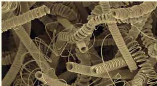
Figure 22: Scanning electron micrograph of carbon microcoils. The coiled fibres range from 250nm–900nm wide. (Image courtesy of AMMRF, University of Sydney)
