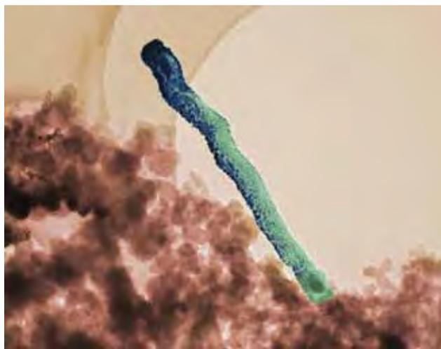
Figure 25: Platinum-coated carbon nanotube for fuel cells (Image courtesy of ANU)
