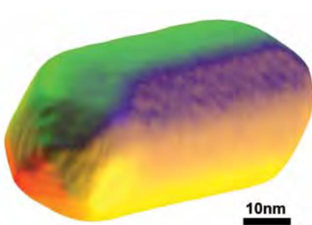
**Figure 7:** Gold nanorods for applications in biosensing. The shape was determined by aberration-corrected electron tomography. (Similar material published in *Nano Letts*, Katz-Boon, H *et al.* (2011) Three-dimensional morphology and crystallography of gold nanorods, 11: 273–278; Image courtesy of Hadas Katz-Boon, Monash University)
