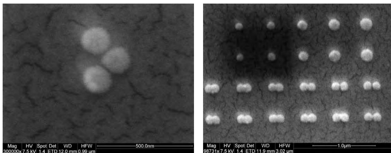
**Figure 41:** The new Melbourne Centre for Nanofabrication, funded by NCRIS, can produce nanophotonic structures by electron beam lithography with spaces down to 5 nm. Here small gold discs exhibit tunable electronic and optical features such as Fano resonances, controlled by the particle size, shape and interparticle spacing. (Image courtesy of Xingzhan Wei, University of Melbourne)
