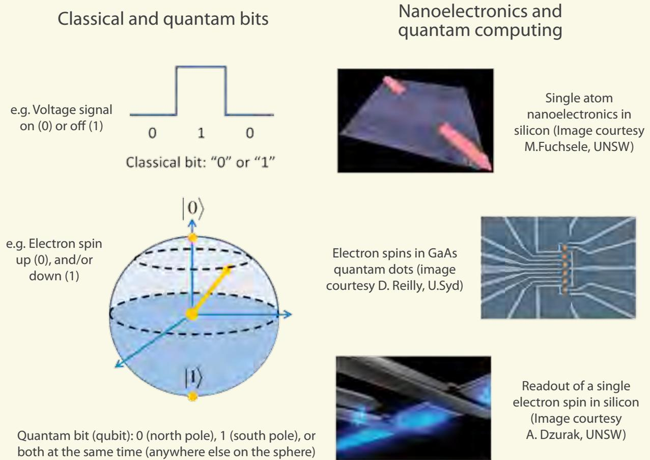
**Figure 2:** Left—The contrast between conventional (classical) information storage using bits and the quantum version—qubits, which allow the two possible bit states to exist at the same time and provide inherent parallelism in information processing. Right—Australian research in quantum computing related to nanoelectronics (see the case study on atomtronics describing approaches based on trapped atoms).
