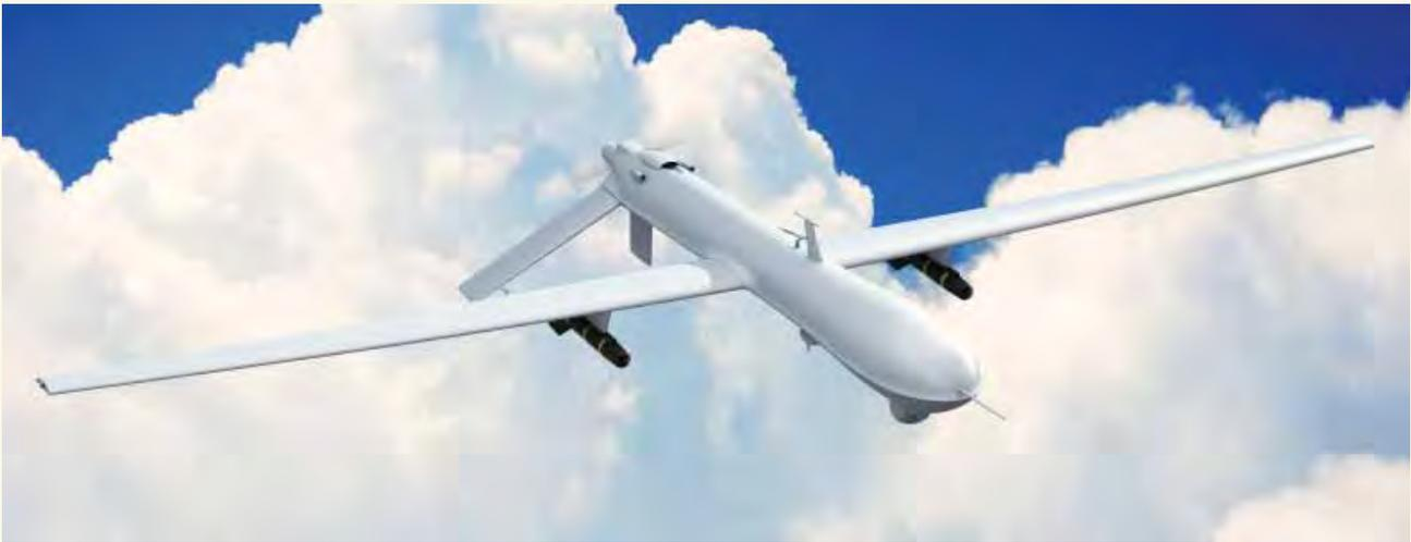
**Figure 43:** Unmanned Aerial Vehicle (UAV) equipped with infrared imaging sensors for intelligence, surveillance and reconnaissance in defence and security applications. (Image: istockphoto.com)
