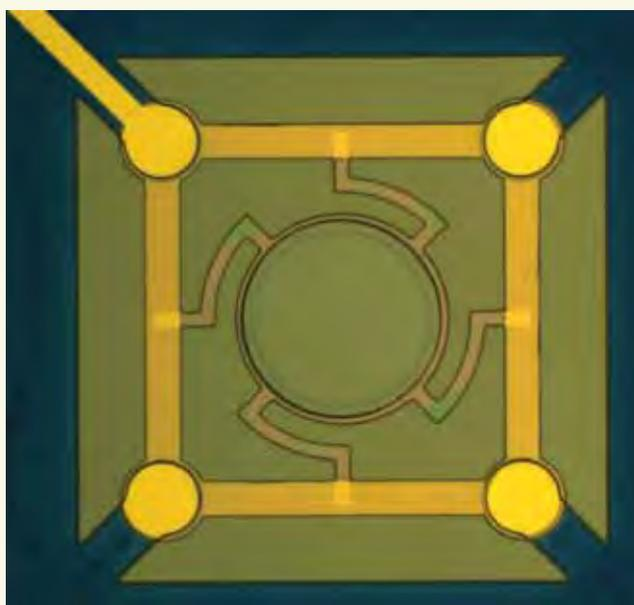
**Figure 42:** Microspectrometer chip for next-generation, wavelength-tuneable infrared imaging sensors. (Image courtesy of MRG UWA)
