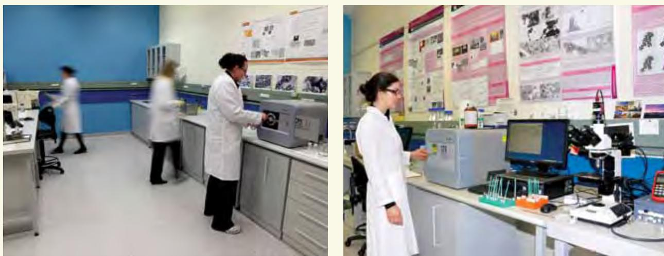
**Figure 48:** Characterising OECD test nanomaterials at the NMI. Left: measuring the aggregation of OECD test nanomaterials using a disc centrifuge in NMI's Nanometrology Section. Right: researchers characterising the physical chemical properties of OECD test nanomaterials using equipment in the NMI's Nanometrology Section. (Images courtesy of NMI)
