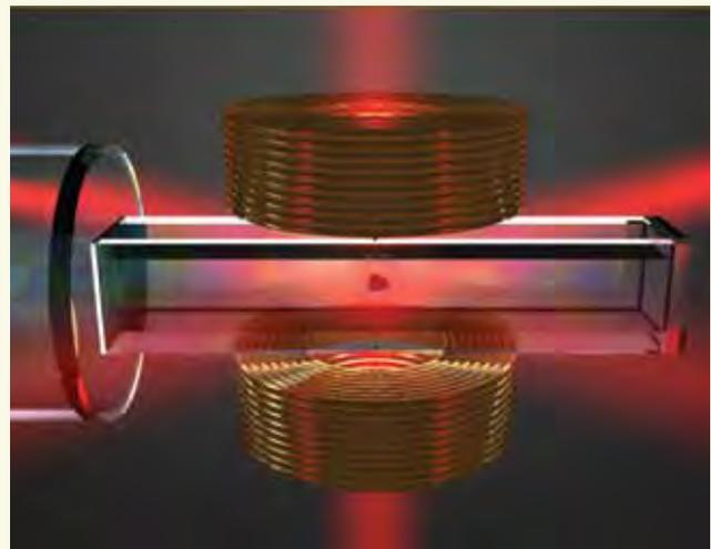
**Figure 40:** Schematic of a magneto-optical trap. Circularly polarised laser beams are shown in red, and a quadrupole magnetic field is produced by two solenoids. Atoms are trapped inside an ultrahigh vacuum system in the centre of the apparatus (Image courtesy of Nick Robins, ANU)
