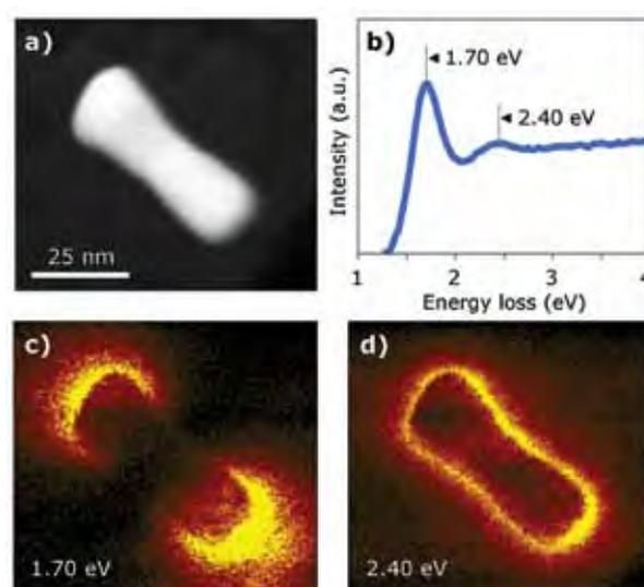
**Figure 10:** Australian researchers were the first to publish maps of surface plasmon excitations in a nanoparticle, in this case, a gold nanorod. (Reprinted from *Nanotechnology* 18 165505 (2007) with the permission of IOP Publishing ; Image courtesy of Vicki Keast, University of Newcastle)
