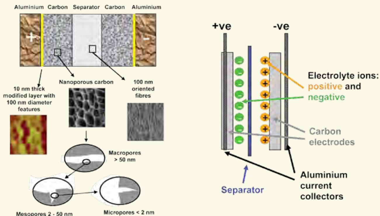
**Figure 32:** Illustration of CAP-XX supercapacitors illustrating the nano-structured materials and interfaces, and a schematic of a CAP-XX EDLC. (Image courtesy of CAP-XX (Australia) Pty Ltd)
