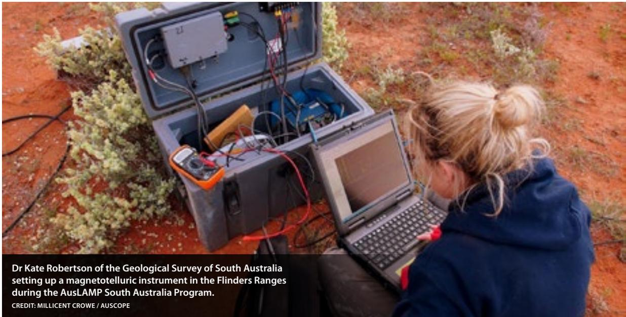
**Dr Kate Robertson of the Geological Survey of South Australia setting up a magnetotelluric instrument in the Flinders Ranges during the AusLAMP South Australia Program.**
