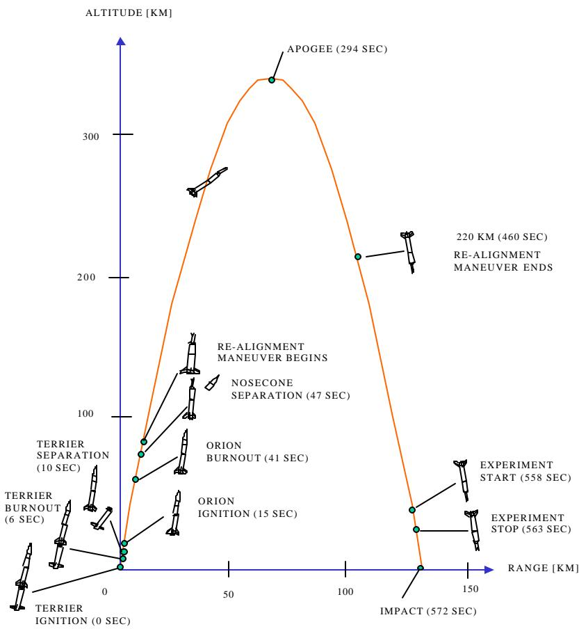
As the combustion process in the scramjet are dependant on the ambient pressure, a highly parabolic trajectory with a near vertical decent during the test time was chosen, so that a correlation could be developed over an envelop of ambient pressures. In addition to the scientific merits, a vertical trajectory is also more cost efficient and there are less structural difficulties resulting from the lower heat and dynamic loads.
